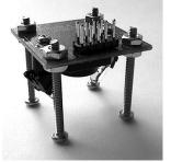
**Figure 2.** Adjustable stand made from machine screws.
