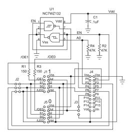
Figure 4. AppMod Adapter Schematic.
