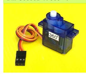
This is a small SERVO MOTOR that can rotate through 360 degrees; it can turn left, turn right and stop without any modifying; so, it is suitably applied to car's wheels, robot's wheels. It uses only 1-Wire I/O for running.
