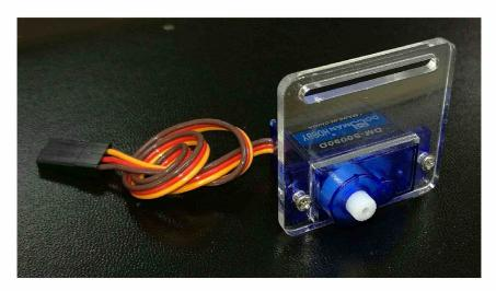
An example shows how to assemble MOUNT SERVO SG90 and DM-S0090D-R-360 SERVO MOTOR.
