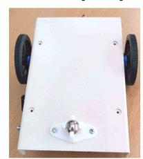
An example shows how to install W420 Ball Wheel as a front wheel of robot.
