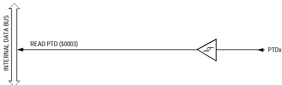
Figure 15-12. Port D Input Circuit
