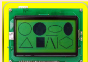
GRAPHIC MODE Can command it to create pictures by self, circle, ellipse, triangle or line
