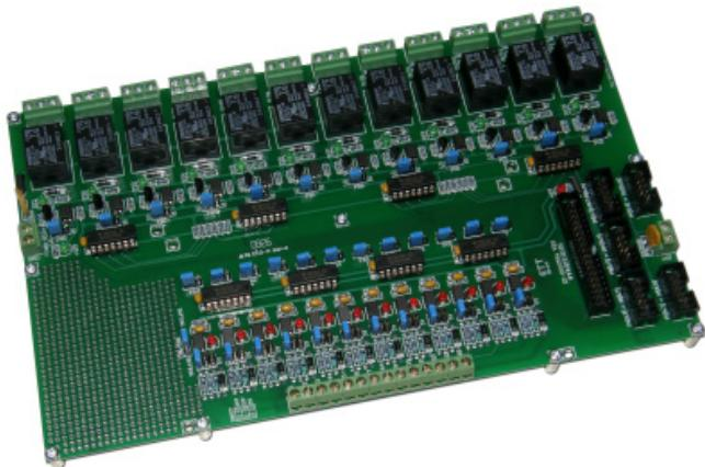
It is the new Board INPUT/OUTPUT Expansion that the replaces ET-INOUT24. It change the Relay size to 10A to use with the higher current; increase the applications of INPUT OPTO for using with INPUT 5V, 12V and 24V; moreover, It increase LOGIC INPUT that is both OUTPUT RELAY and INPUT OPTO, so user can select LOGIC to run either as LOGIC LOW or as LOGIC HI.
