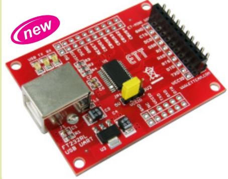
It is Board that converts signal from PORT USB of computer to be UART Serial in the format of Signal TTL; so, it is suitable for directly interfacing with Board Microcontrollers.
