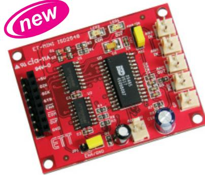
ET-MINI ISD2548 is MINI Board that records sound and playback; it is suitable for recording sound that is not longer than 48 seconds. It controls record and playback by interfacing with MCU in the format of SERIAL DATA (SPI) through IC 74HC595 to reduce amount of Pin I/O of the connected MCU.
