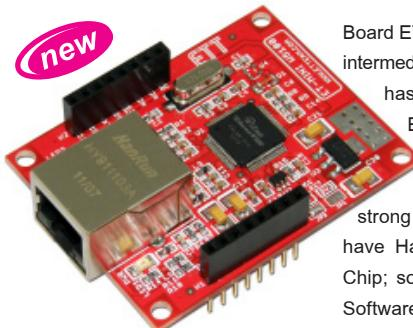
Board ET-MINI W5100 is designed to be intermediate between Microcontroller that has no any PORT Ethernet and Ethernet Network. This board uses Chip Ethernet Controller No.W5100 from WIZnet. The strong point of this Chip number is to have Hardwired TCP/IP stack internal Chip; so, it isun necessary to write any Software TCP/IP Stack from external. It is easier to use and it does not waste much resource of the connected Microcontroller.
