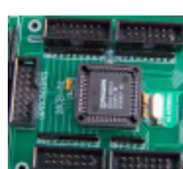
CPU MCS-51 OF ET-LAB3A AS NO. P89V51RD2 WITH 64 KBYTE INTERNAL FLASH MEMORY
